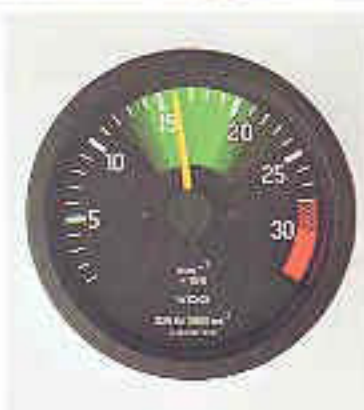
The green zone, always in view, is an important aid to economical driving.
