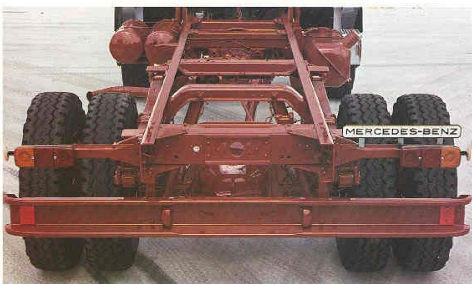
The frames for drop-siders and dump trucks are made of sturdy U-section longitudinal members to which cross-members are riveted to give high torsional flexibility. The front cross-member takes the coupling jaw and pin. The rear cross-member can be fitted with a trailer coupling. Engine and gearbox are suspended on rubber vibration dampers. The special double frame of the semitrailer tractors is reinforced by L-shaped longitudinal members. This considerably improves torsional resistance.
