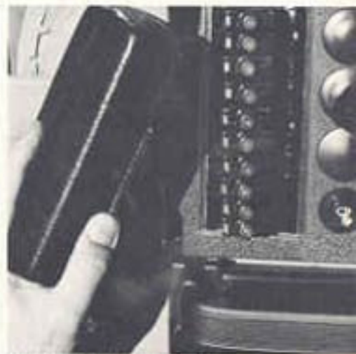
Instead of fuses, circuit breakers are conveniently positioned on the dashboard.
