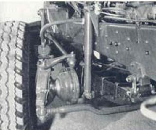
The front springs are 1,000 mm long. Both rear leaf springs are mounted to the frame in the spring center. The free ends rest in guides on the rear axle. The rear axle suspension is designed to permit a very low to give the springs their central point a turning angle of 15 degrees to both sides. The relatively large movement of the rear rear axle considerably improves the cross-country mobility.
