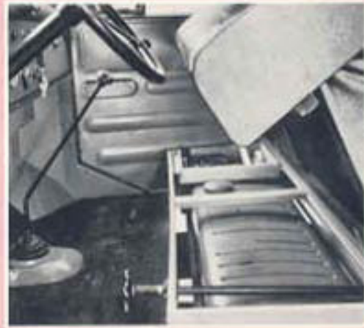
The fuel tank holding six gallons is placed under
