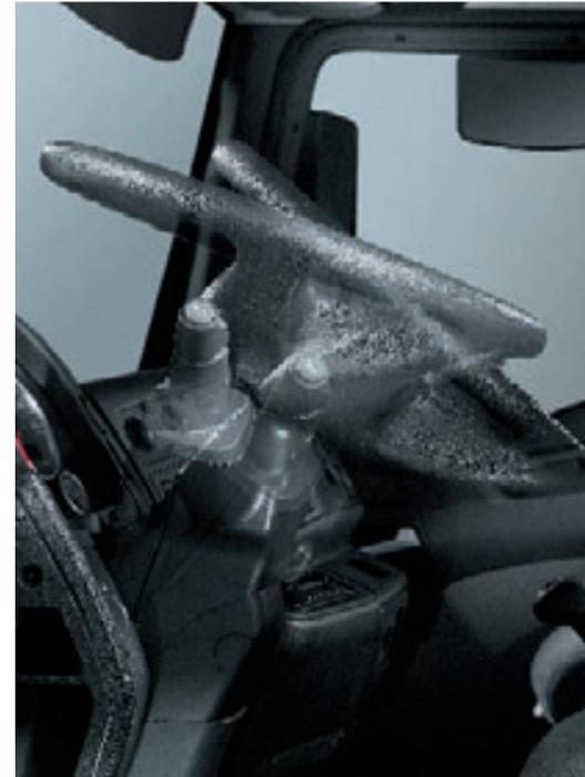
Multifunction steering wheel with controls for functions including MAN radio and cruise control, standard in the L and LX cabs.
