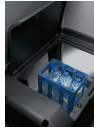
Large storage compartment in L and LX cabs, accessible from inside and outside the cab.
