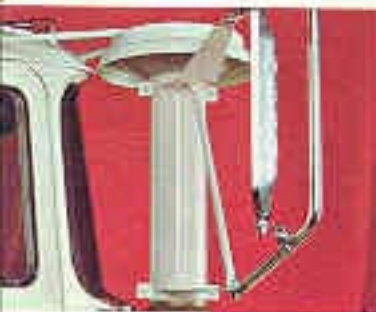
5. Air intake—positioned 23 inches above the extra-large cleaner. In rain, an auxiliary intake under hood is used.
