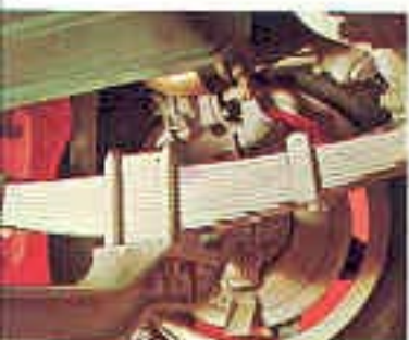
9. Front springs—are 54 inches long; 3 1/2 inches wide for softer ride. Wood spring centers cut tendency to sway.
