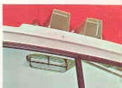
4. Comfort control—the Mack U has a new two-way roof ventilator and central heating system to provide exact comfort control in any driving weather.
