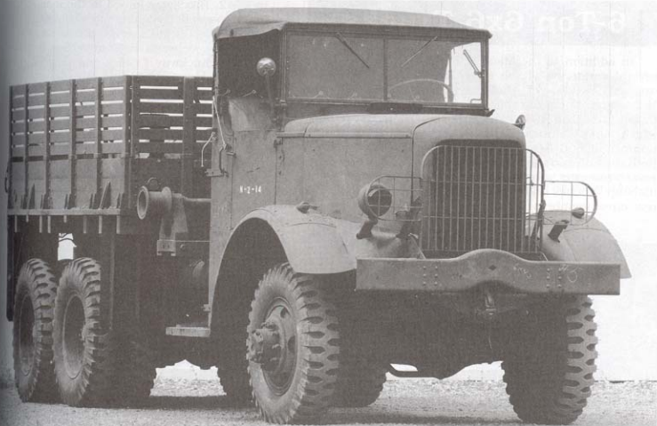
In 1944, this NM-7 posed for a portrait at the Studebaker Proving Ground. The capstan head for the midship winch is clearly seen. The spare tires for the NM were carried in the truck bed. (U.S. Army photo)
