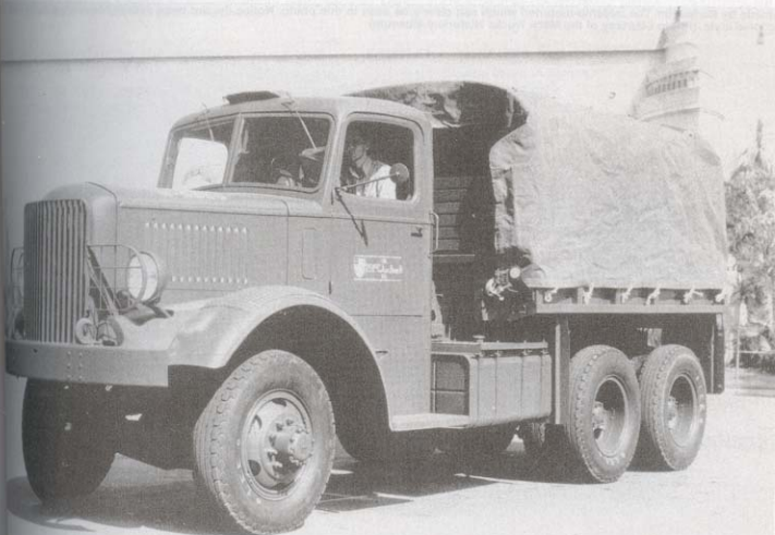
The NM-1 (shown here), NM-2, and NM-3 trucks were supplied with Lee tires with highway tread. Initially, the size was 9.75 x 22 in., but soon that was changed to 10-22. The NM-1 and -2 had a flat bumper with tow hooks mounted on the top. (Photo courtesy of the Mack Trucks Historical Museum)
