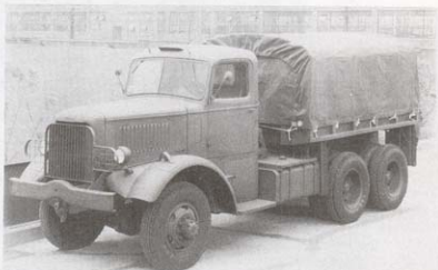
The NM series trucks were tall. The hardtop versions stand just over 9 ft. to the top of the cab. The cargo beds of the NM-1 through -3 were steel, and built by Perfection. Beginning with the NM-3, the front bumper, now sans tow hook, was arched to clear a pintle hook mounted on the front cross member. Also, the brush guard of the NM-3 and later trucks was considerably smaller than on the earlier trucks. (Photo courtesy of the Mack Trucks Historical Museum)
