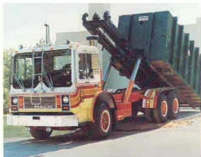
For high-cube roll-off loads, the MR has deep-section frame rails and other heavy-duty components to provide strength and durability.
