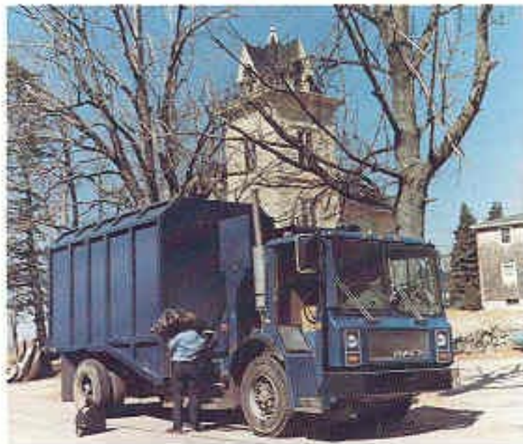
The Mack MR adapts easily to most body configurations, including this side loader. One-man stand-up drive and pick-up from the right side; left-hand drive to the landfill.
