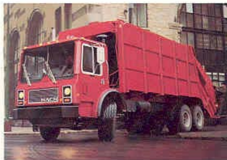
With the rear loader body, the MR is one of the best all-around, heavy-duty refuse units in the industry. A wide range of PTO requirements can be accommodated with either the Mack full-time flywheel power take-off or one of the rear- or side-mounted power take-offs.
