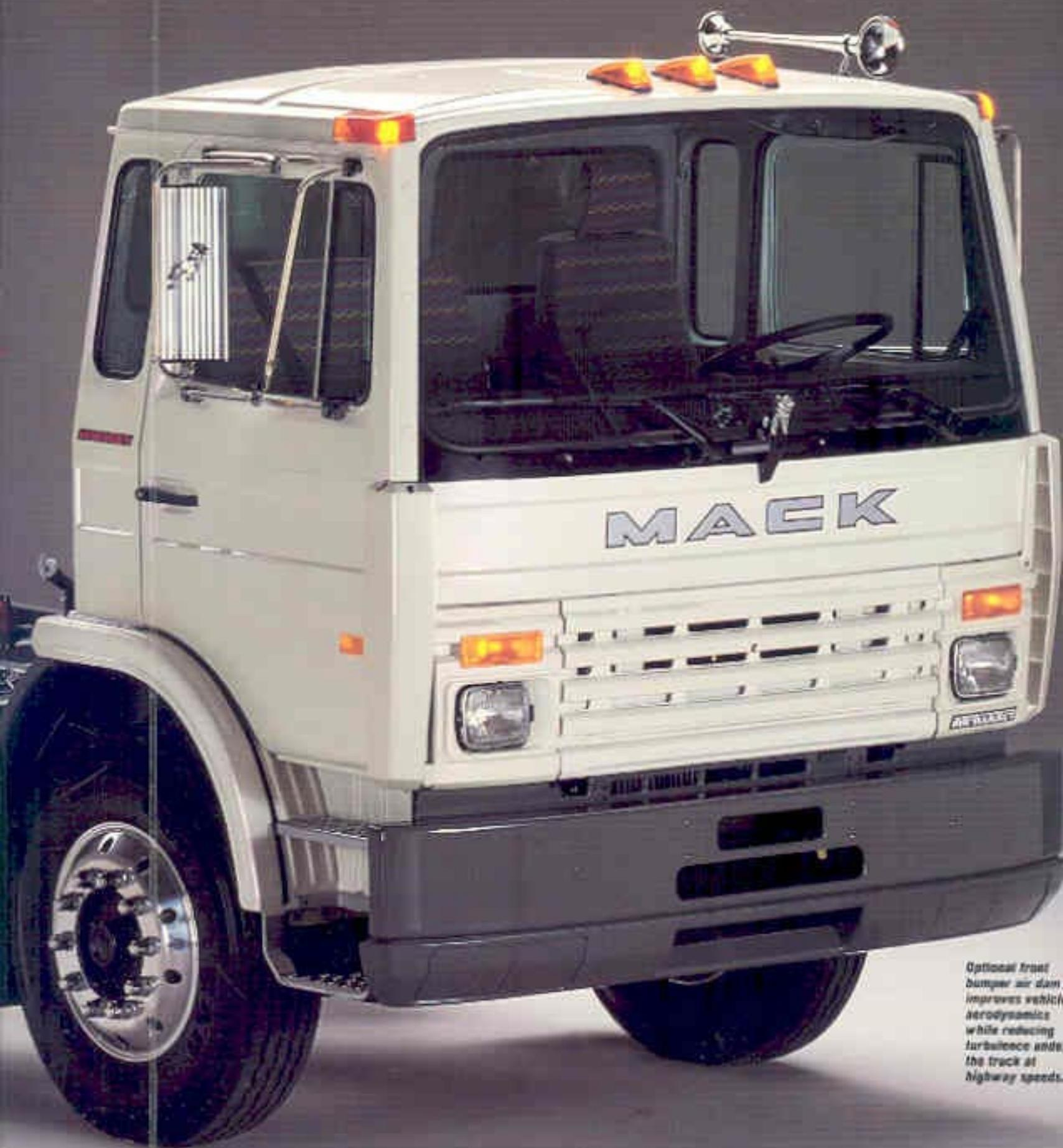
*Optional front bumper air dam improves vehicle aerodynamics while reducing turbulence under the truck at highway speeds.*
