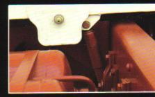
The Mid-Liner CS cab is suspended with shock absorbers and rubber insulators at all four mounting points for soothing comfort in punishing day-to-day service.
