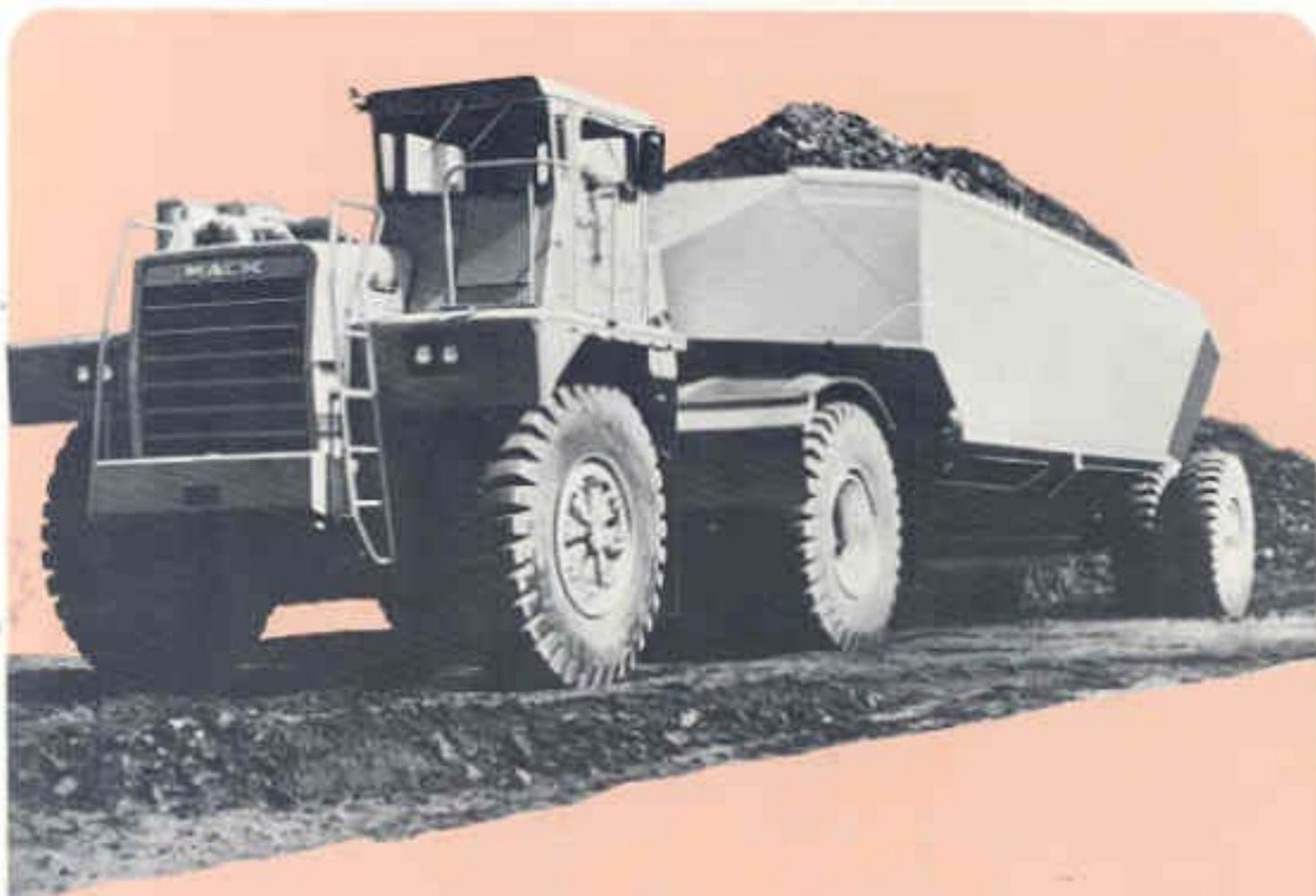
MACK traditional dependability and long history of off-highway manufacturing skill are proof of cost-cutting performance by this 120-ton, Mack four-wheel tractor with bottom dump type semi-trailer.
