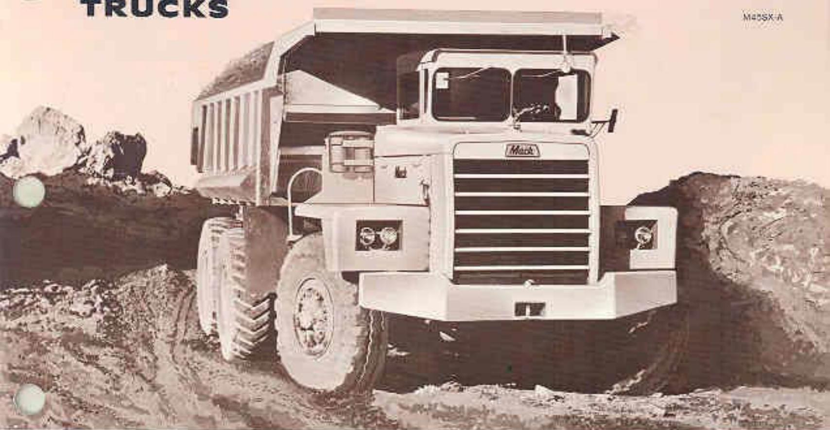
Mack Model M-45SX is a diesel powered six-wheel, end-dump truck that is setting new standards in efficient, low cost haulage of increased payloads in demanding off-highway service. This huge Off-Highway Mack, with its great tractive ability, is an ideal large pit, quarry and general excavation transport.
