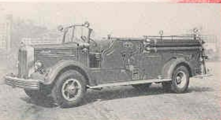
Type 19, 1000-gallon, triple combination pumping engine with standard open seat.
