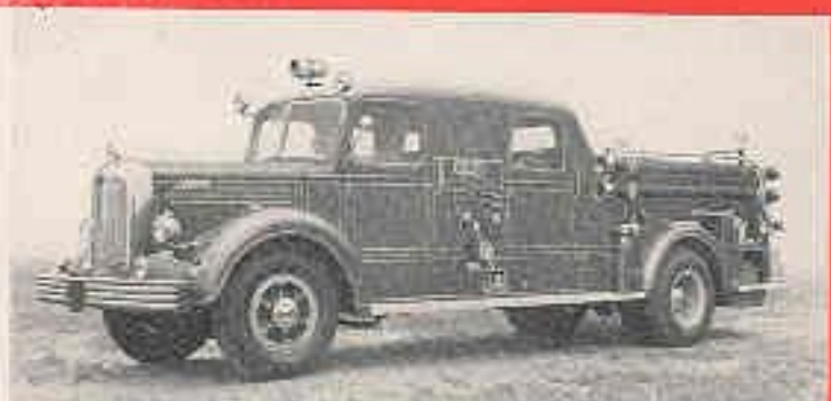
Type 19, triple combination pumping engine with special seven man sedan type cab.
