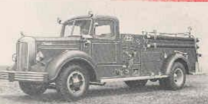
Type 19, 1000-gallon, triple combination pumper with closed cab.
