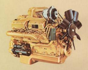
The Maxidyne V-8 325 hp (242 kW) diesel (ENDT 865) creates high torque at low RPM, producing nearly constant horsepower over a wide operating range. The high-torque-capacity Maxitorque transmission (TRDL 1070) is specifically designed to work with the high-perfor-
