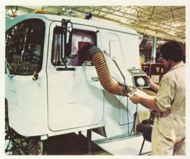
Cabs are pressure-tested for proper sealing. Sealing keeps out noise, fumes, heat, cold and moisture.
