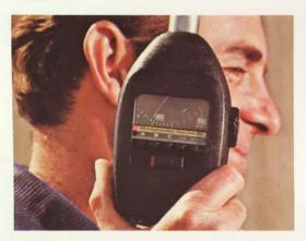
Mack trucks are designed to be quiet. Interior sound levels are well below BMCS specifications. A special compound applied to the floor to prevent rust, also helps deaden noise.
