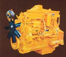
Cat 3406 is a big-bore diesel available in both high-torque-rise and conventional-torque-rise versions, with horsepower from 280 (209 kW) to 360 (268 kW).
