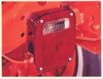
Rear lights combine tail, stop, directional and back-up lamp functions in one unit. Water-tight design eliminates internal corrosion and resultant breakdown of the electrical system. Bulbs are shock-mounted to reduce filament breakage.
