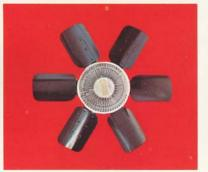
The variable-speed fan drive operates on demand when cooling is needed, reducing parasitic power losses, saving fuel, and lowering noise levels.
