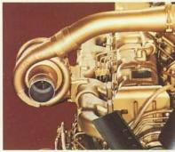
Turbochargers, standard on all Mack engines to increase horse-power, also serve as effective noise-muffling devices.
