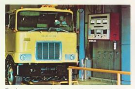
Engines, transmissions and axles are dynamometer-tested for noise, leaks and vibration.
