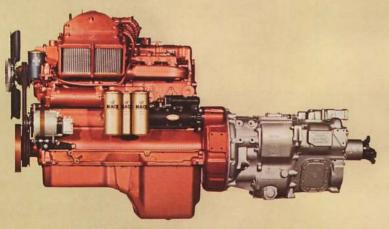
Mack's sensational "300-PLUS" engine (ETAZ 673A), introduced in late 1975, is a modified high-torque-rise version of the 300 Series engine. Developing 315 hp (235 kW) at 1900 RPM, its torque curve has been tailored for a traditional 10-speed transmission . . . yet it produces almost as much torque (1050 ft/lbs (1 424 Nm) at 1450 RPM) as its
