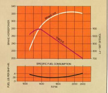
mance Maxidyne. The unique ability of this engine-transmission combination to operate with only five evenly-spaced gears results in less shifting, faster acceleration, higher average road speeds, reduced trip time, and fuel savings.
