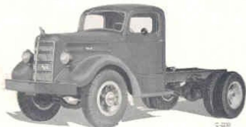
**S**PECIFICALLY designed for tractor service alone, this model is a companion to the Model EG chassis and follows generally the same make-up of components, using the same thrifty, yet energetic engine of 330 cu. in. displacement. It has its own frame, especially braced for fifth-wheel load, with Mack's exclusive box-girder cross-members, somewhat larger brakes, Hydrovac operated, and longer front springs.
