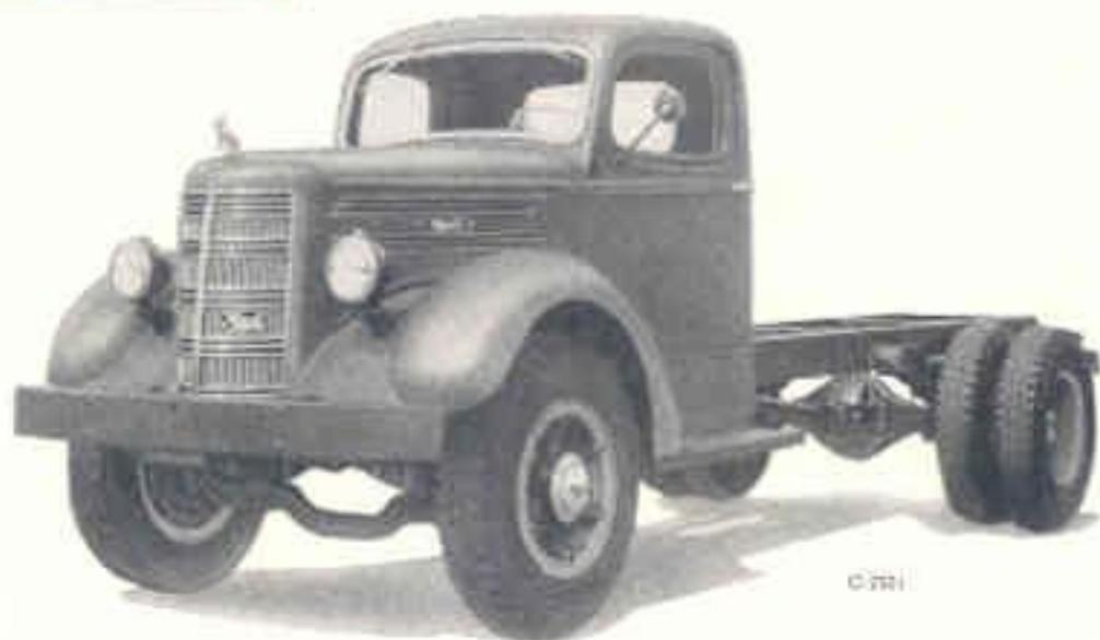
**F**OR those services which lie between the medium and heavy classes of chassis, the Mack Model EG has been created. Responsive performance is attained through an extremely efficient engine of 330-cubic inch displacement. Power is transmitted to either a Single-reduction or Dual Reduction rear axle through a five-speed transmission or, where needed, the sensational 10-speed Mack Mono-shift Duplex type.
