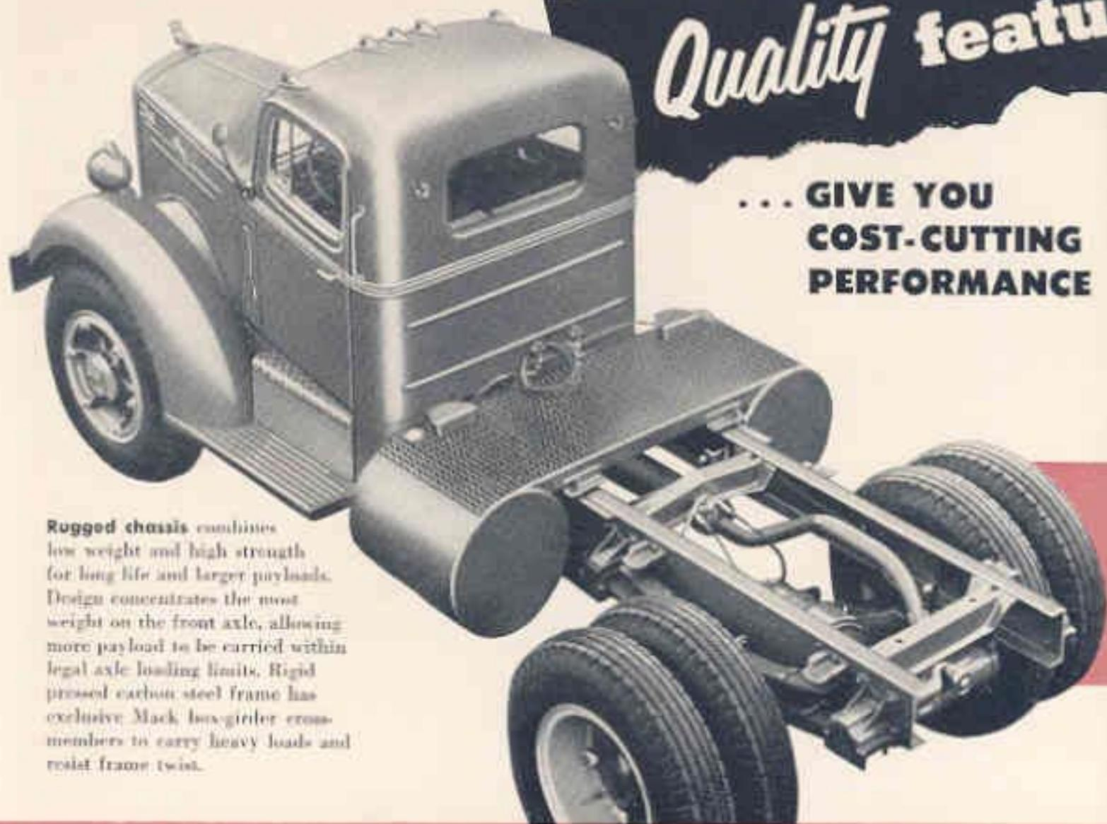
**Rugged chassis** combines low weight and high strength for long life and larger payloads. Design concentrates the most weight on the front axle, allowing more payload to be carried within legal axle loading limits. Rigid pressed carbon steel frame has exclusive Mack box-girder crossmembers to carry heavy loads and resist frame twist.
