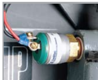
Screw on terminals don't shake loose.
