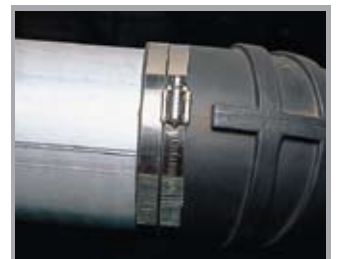
Double clamping provides extra engine protection.
