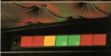
MAJOR WARNING LAMPS ARE LOCATED ABOVE THE VISOR SO YOU CAN KEEP AN EYE ON AIR, OIL, COOLANT AND OTHER MAJOR SYSTEMS WITHOUT TAKING YOUR EYES OFF THE ROAD.
