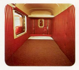
The Conventional sleeper compartment is completely rolled and padded on all wall panels. The headliner is of the same molded Cycolac material as in the cab, textured to enhance the beauty of the Splendor Interior. The doors at each end of the sleeper are rolled and padded with tight-sealing vents for added comfort.
