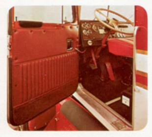
The Splendor Interior door pad is rolled and padded with the lower kick area completed in coordinating colored nylon carpeting for extended wear, ease of cleaning, and outstanding appearance. Window roll down handles and flush mounted door latch handles are finished in high gloss chrome and along the window ledge is a black vinyl padded arm rest.
