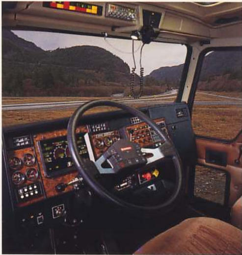
Kenworth's exclusive SmartWheel puts 11 of the most frequently used controls — including engine retarders, cruise control, headlight and marker light flashers — right under the driver's fingertips.
