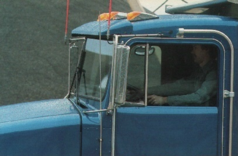
FLAT GLASS IN THE WINDSHIELD HELPS ELIMINATE DISTORTION AND IS FASTER, LESS EXPENSIVE TO REPLACE.
