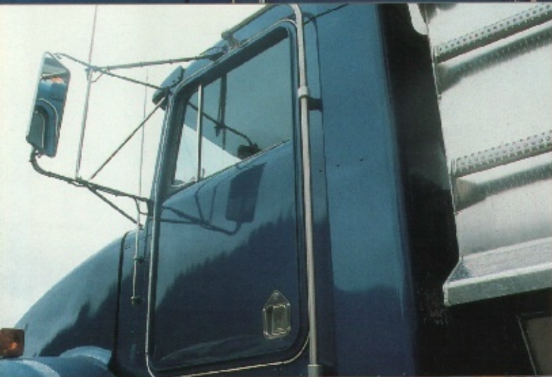
LOW, PULL-TYPE DOOR HANDLES AND OVERSIZED CAB-MOUNTED GRAB HANDLES MAKE IT EASIER TO GET AND OUT OF THE CAB.
