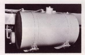
Fuel tanks are side-mounted on the frame. At Kenworth you may choose from varying capacities and locations.
