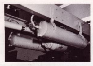
Dual reservoir tanks of ample capacity help to make Kenworth braking the safest, fastest acting, most trouble-free available.
