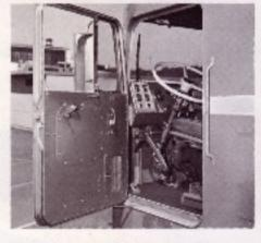
Bulkhead door features continuous door frame and weather stripping, plus piano-type hinges.
