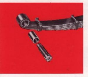
Threaded steel-to-steel pins and bushings in front springs last longer, eliminate side movement.
