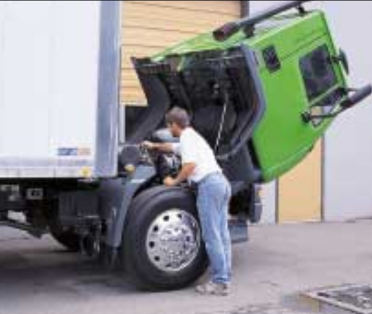
Tilting the cab a full 60 degrees for complete access to the engine compartment is virtually effortless.
