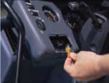
An easily accessed fuse panel, located inside the cab, centralizes all circuit protection elements.
