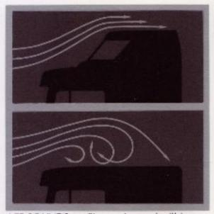
AERODYNE'S roofline acts as a built-in wind deflector that reduces turbulence associated with standard COE designs to reduce drag, cut fuel consumption and relieve some of the strain on the engine and drive train.
