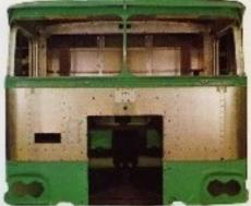
The Kenworth cab is a carefully engineered combination of aluminum and fiber glass. In case of accident, damaged panels are easily replaced.
