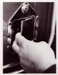
Redesigned pull-type flush mounted door handle is placed low on outside of door so that it can be easily reached from the ground. Same key that opens the door operates the engine switch.
