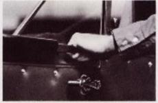
One-piece, full-width aluminum casting strengthens the door and forms an integral grab handle and arm rest. Another example of superior design to give you a better truck at no extra cost.
