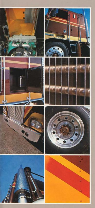
The **engine tunnel** is a single fiberglass unit that's insulated to reduce cab noise and improve temperature control.
