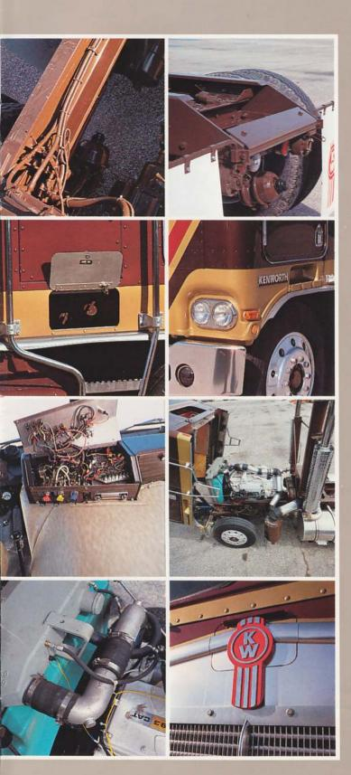
**Air and light lines** are tightly bundled and mounted high off the flange to avoid moisture, road salts and dirt.
