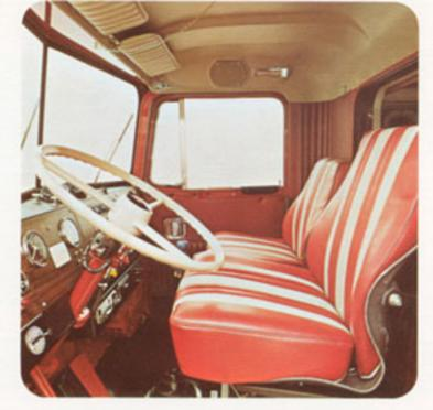
This conventional cab is appointed with the Splendor Interior. The Splendor seats, door pads, and back panels are rolled and padded for outstanding and tasteful appearance as well as comfort and luxury. The Splendor material is rugged expanded vinyl, stitched with extra strong dacron thread. The head-
