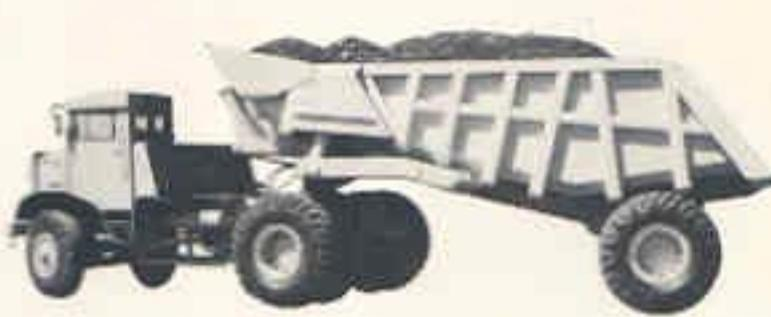
**802-B DUMPING ACTION** moves the tractor backward and under the trailer, while the entire trailer raises. Kenworth's rugged pin-type construction of the fifth wheel insures excellent stability both in dumping and over the road hauling. A special guide and equalizer stabilizes the body during dumping. The hoist mechanism is the same as on other Kenworth rock and ore movers.
