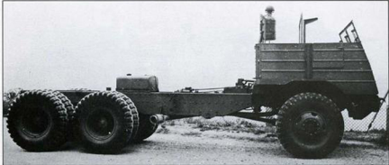
Chassis/cab of the unarmoured Kenworth 580. Note the elevated position of the engine air cleaner.
