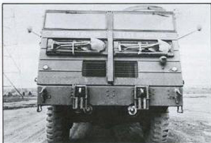
Front views, stages 1 and 2. The second picture also shows the double air intake grilles, a later modification.
