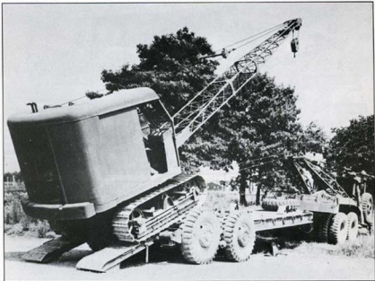
Loading a crawler-mounted crane onto the experimental 20-ton Ordnance trailer at Fort Knox. The trailer is attached by a Mack coupler.
