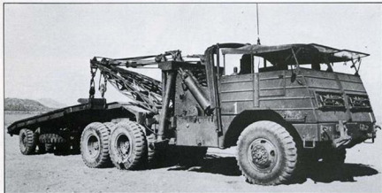
The soft-skin Kenworth 580 complete with recovery semi-trailer. This picture shows the vehicle as originally delivered (with fifth wheel couplings) and was taken during the initial tests at the Desert Warfare Board, Camp Young, California. The large number '1' on front and sides probably correspond with the '2' on the Ward LaFrance (see page 18.)
