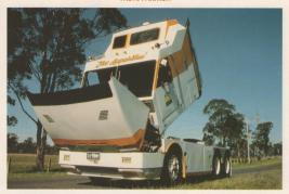
by no means overweight, as one might expect of a home-brewed wagon. The rig tares off at 8.94 tonnes, or half a tonne lighter than a W900 Kenworth Aerodyne.
