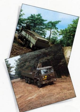
DAF YAZ 2300 general purpose vehicle, payload 10 tons, 6x6, 24 V designed and built in accordance with the latest requirements and chosen as the standard heavy transport vehicle for operation with the Dutch Armed Forces.
