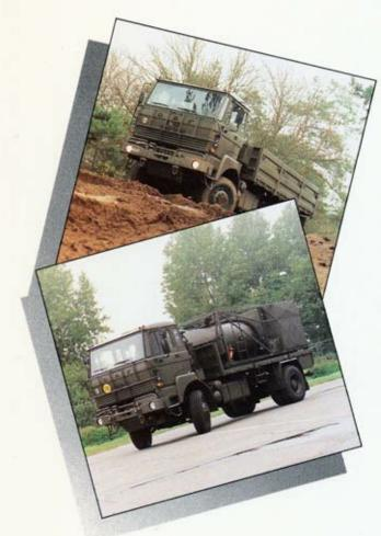
DAF YAV 2300 general purpose vehicle, payload up to 7 tonnes, 4x4, 24V, designed and built in accordance with the latest requirements and chosen as prime mover for AFCENT's alternate war headquarters.
