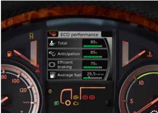
**INFORMATIVE** The DAF Driver Performance Assistant (DPA) helps the driver to drive as economically as possible. The central color display informs about fuel consumption, braking behaviour, anticipation of traffic situations and shows the optimal moment for gear changing. Useful are tips for saving fuel, optimum use of the engine brake and the importance of the right spoiler adjustment and tyre pressure. The DPA motivates the driver to get the best from the XF with minimal effort.
