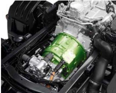
Between clutch and gearbox is the electric motor which provides drive as well as a generator function
