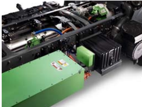
Energy released during braking is stored in special lithium-ion batteries
