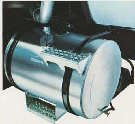
Aluminum fuel tanks. Dual 75-gallon fuel tanks and brackets are available. They meet ICC specifications.
