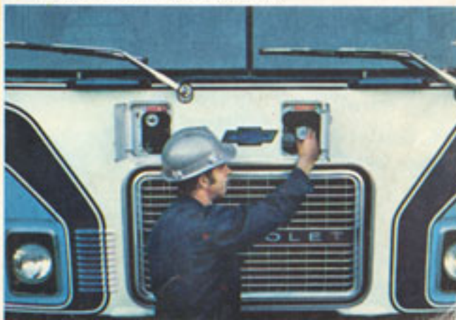
Hydraulic tilting mechanism. Water and oil fill access doors.
