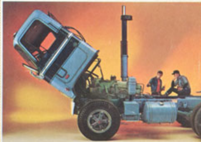
Hydraulic tilting mechanism. Water and oil fill access doors.
