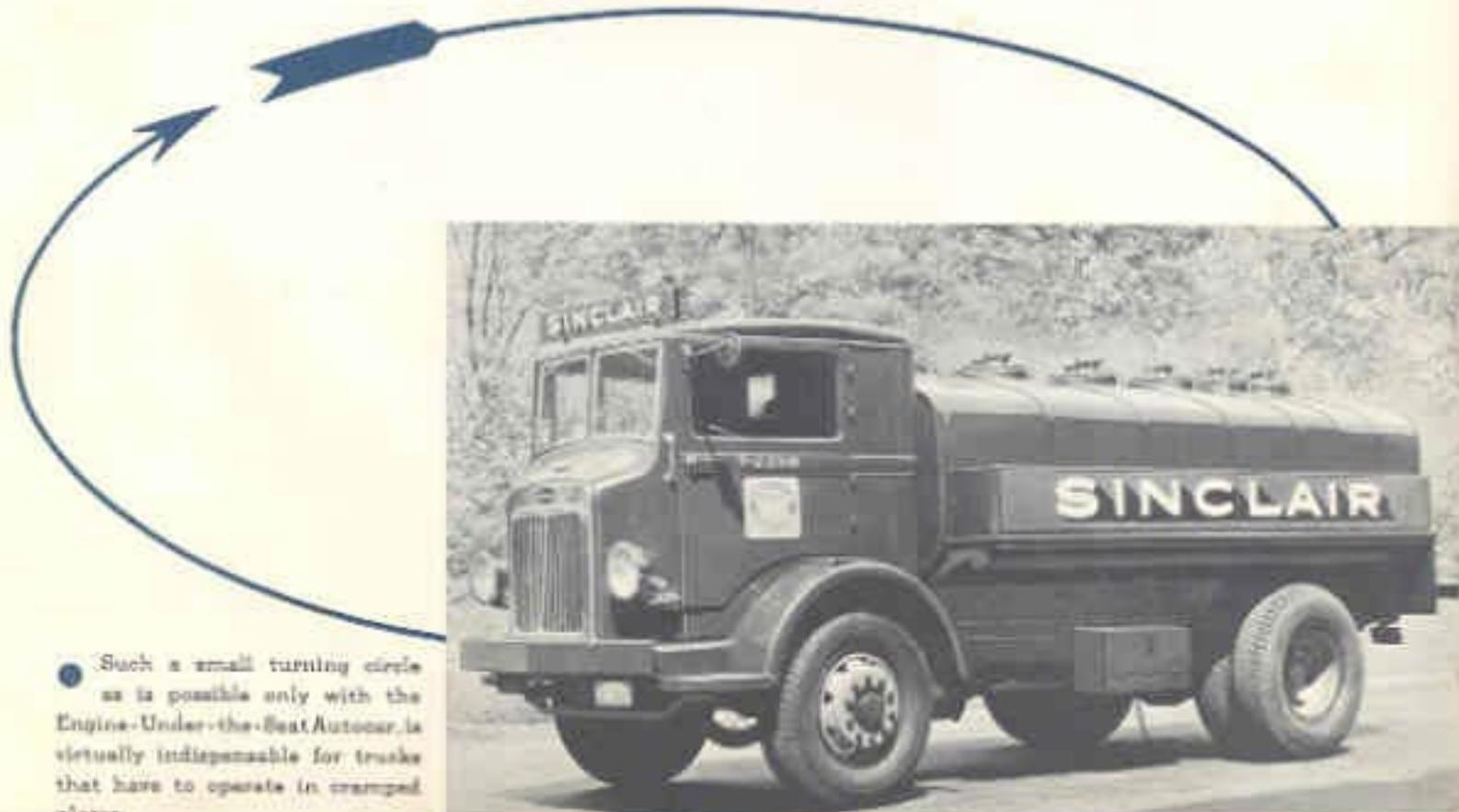
Such a small turning circle is possible only with the Engine-Under-the-Seat Autocar. It is virtually indispensable for trucks that have to operate in cramped places.
