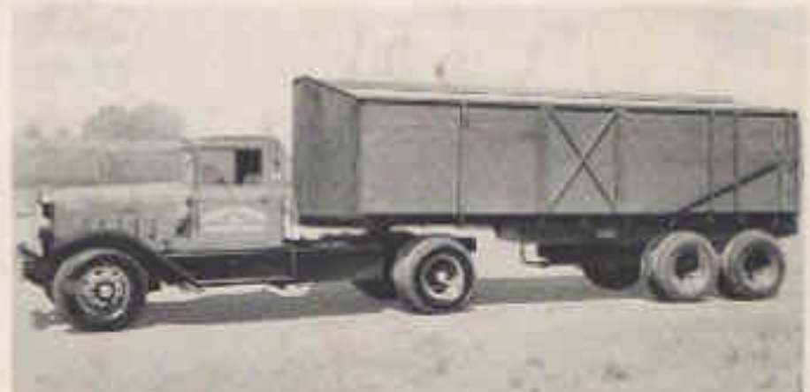
Built to comply with the laws of both California and Oregon, this Autocar-Diesel tractor's 22-foot trailer has a five-foot tail gate which can be lowered to carry additional all drums. It is owned by Contract Carriers, Inc., Fresno, Calif.
