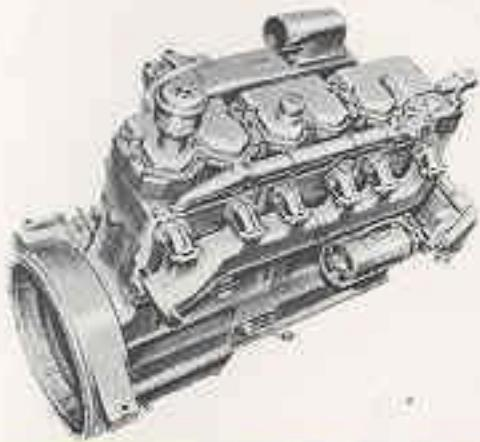
**AUTOCAR-CUMMINS DIESEL ENGINES.** Engines for the DC 103 D-OH Planetary Packaged are the Cummins 6-cylinder, valve-in-head diesel known by engineers the world over for quality, ruggedness, and long operating life. Operators are offered as standard the NT engine delivering 220 hp at 2100 rpm. Optional equipment is the NT with 250 hp or the NTO with 262 hp.
