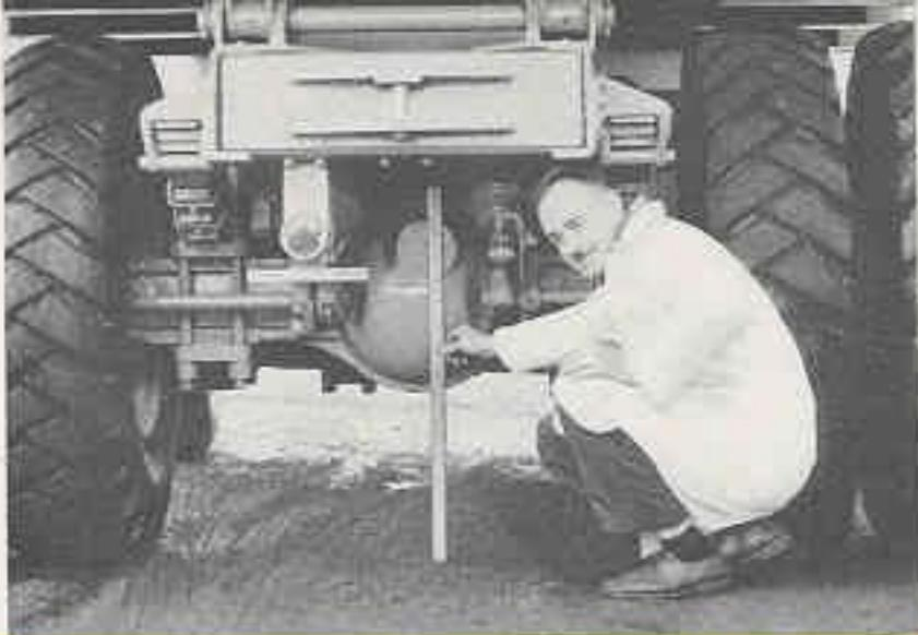
**THE PLANETARY GEAR REAR AXLE** places the highest numerical gear reduction right in the wheels. This means that axle shafts and hypoid gears carry only nominal torsional loads and give long trouble-free service. Extra long life, extra dependability, extra economy.
