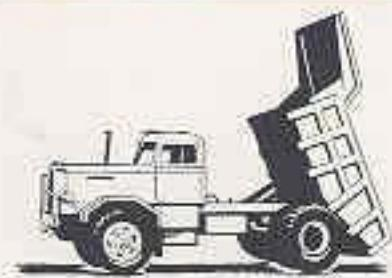
**70° DUMPING ANGLE** provided by double-acting hydraulic hoist.
