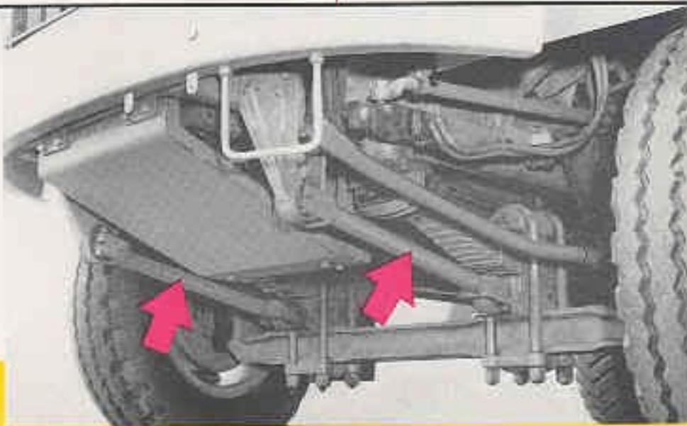
**HEAVY-DUTY RADIUS RODS,** front and rear, hold axles in alignment with frame, provide the rigid construction that reduces stresses.
