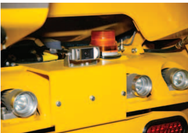
The MT5020 is standard equipped with a rear vision camera. A small detail, but definitely worth viewing - is the standard equipped camera for improved operator's visibility.
