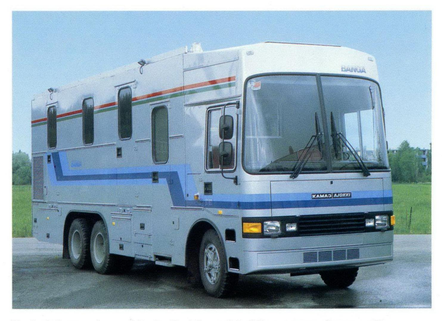
The body is manufactured by the Finnish coach-building company Carrus and is designed to meet the specifications by the TV-broadcasting equipment producer Banga. The body has efficient sound and thermal insulation and is equipped with air conditioning and heating systems. All this provides the possibility to operate in climatic conditions from – 40 C up to +40 C and still have comfortable conditions for the occupants in the unit.
