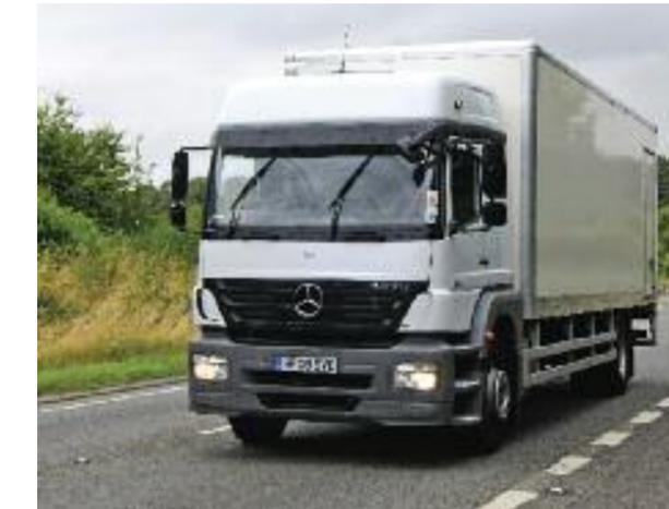
Axor also brings another key benefit to urban operations as well - the MSS engine start/stop system which switches off the engine when the vehicle is waiting in traffic. Offered as standard in the UK with all Axor 6.4 and 7.2 litre engines, MSS cuts the engine if the vehicle is stationary, in neutral gear and the clutch pedal not being operated. Instant restart occurs when the clutch pedal is depressed and a gear selected prior to moving off.
