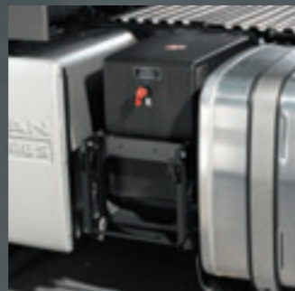
Compact battery box.
