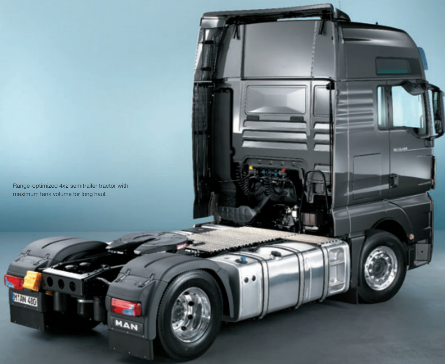
Compressed air tanks situated at the rear.
