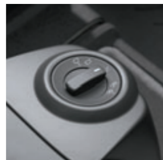
MAN TipMatic® rotary switch.
