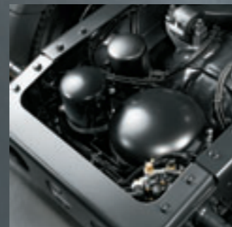
Compressed air tanks situated at the rear.
