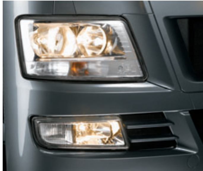
Headlights with free-form reflectors, Xenon dipped light.
