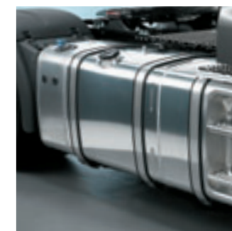
Combination tank for diesel and AdBlue®.
