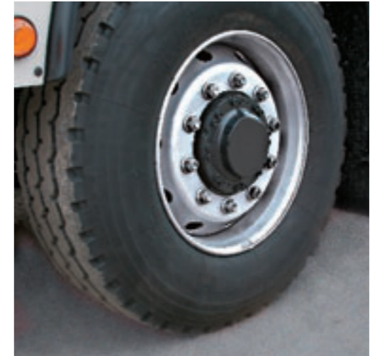
MAN HydroDrive® wheel hub motor.
