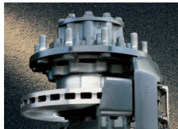
Disc brakes with hypoid and steering axles.
