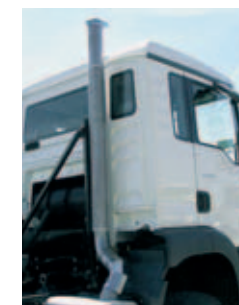
Vertical exhaust pipe.
