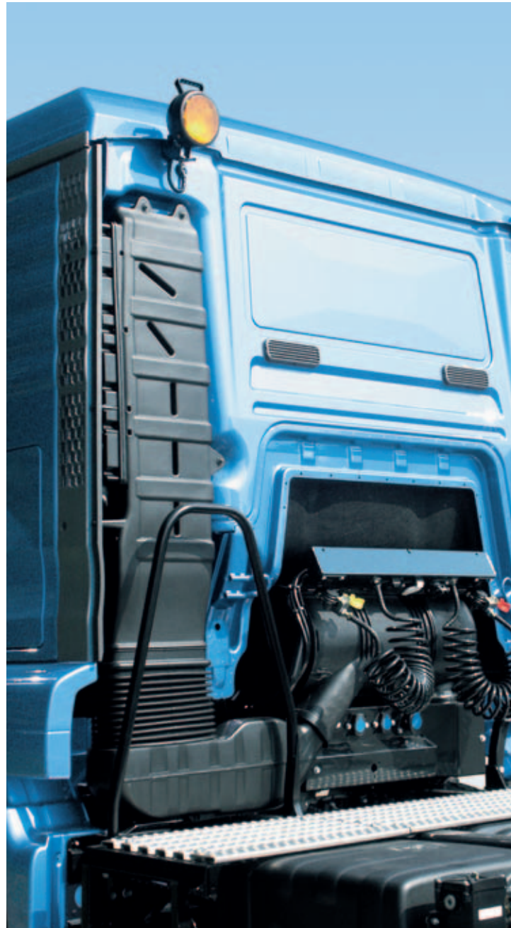
Elevated air intake.
