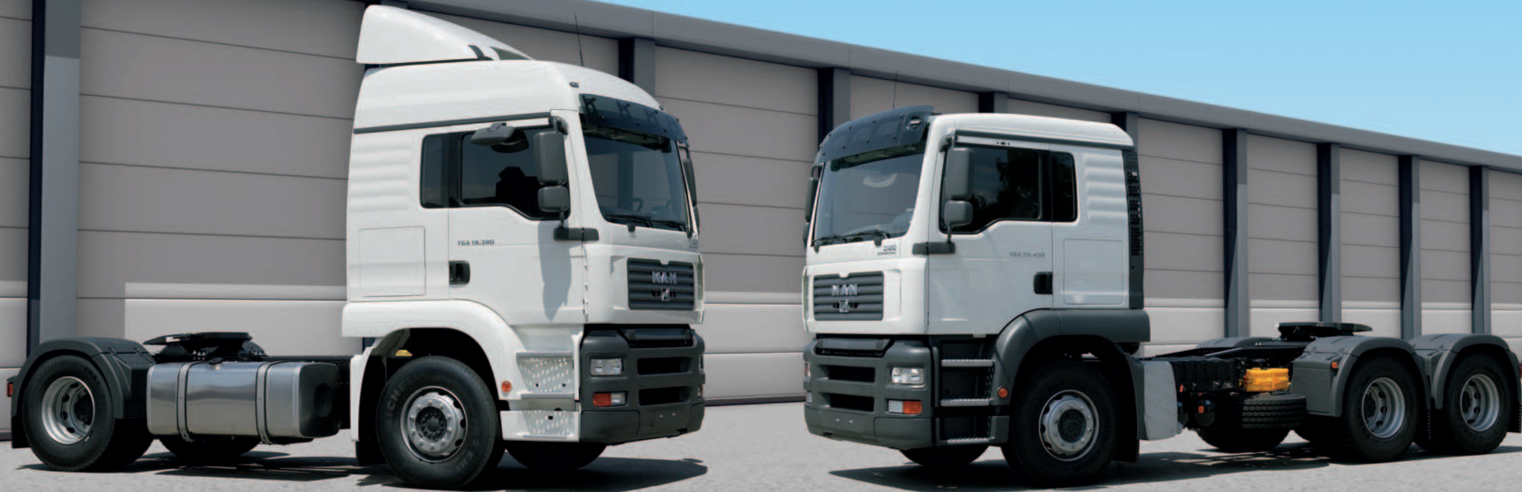
Semitrailer tractor 4x2, leaf/air suspension.
