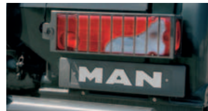
Headlights and rear lights with swivel-mounted stone-chip protection.
