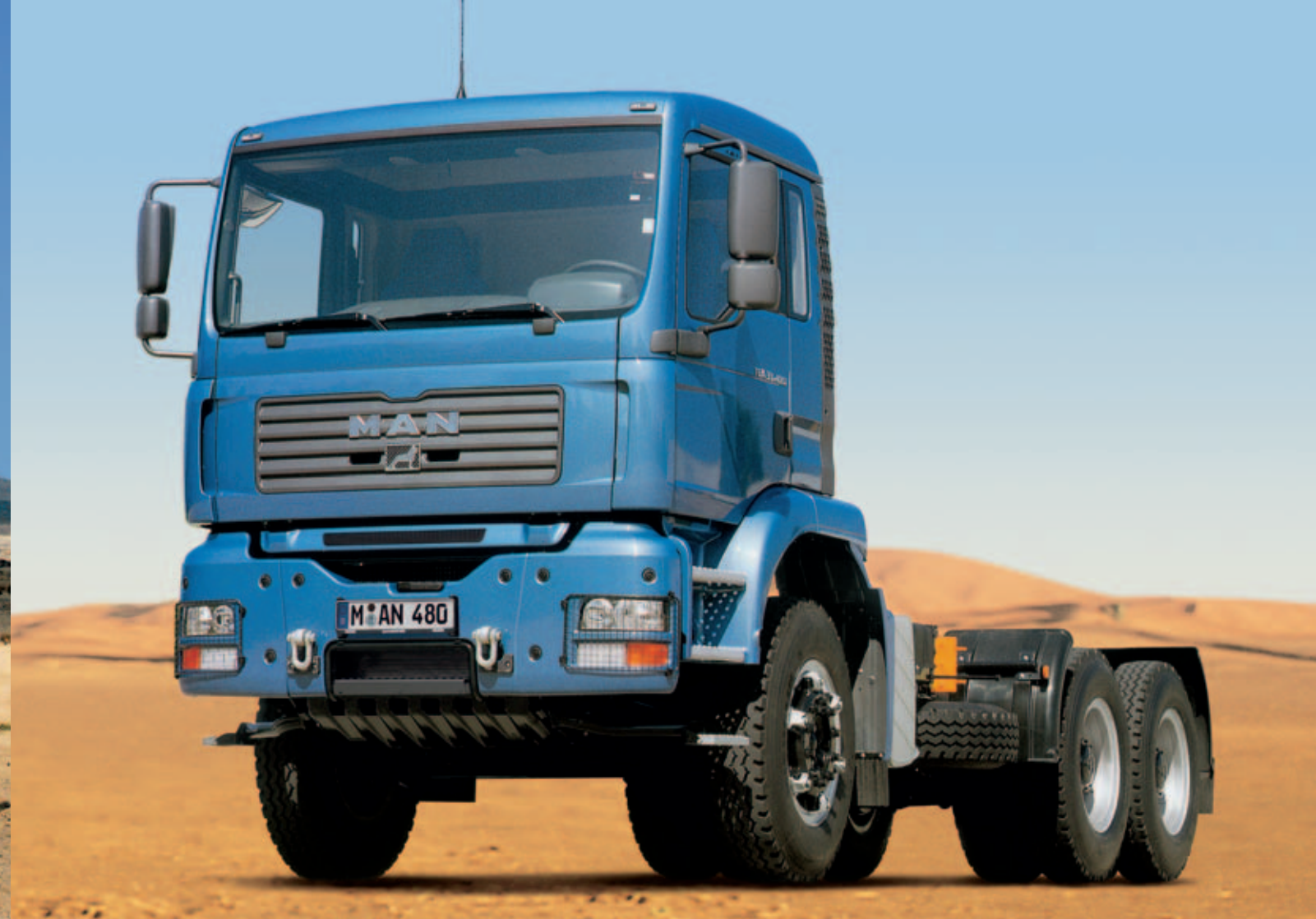
Chassis 6x4 with leaf suspension.
