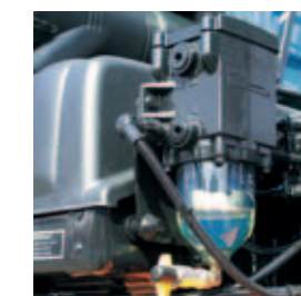
A Separ fuel filter is part of the standard delivery, while a heated version is an option
