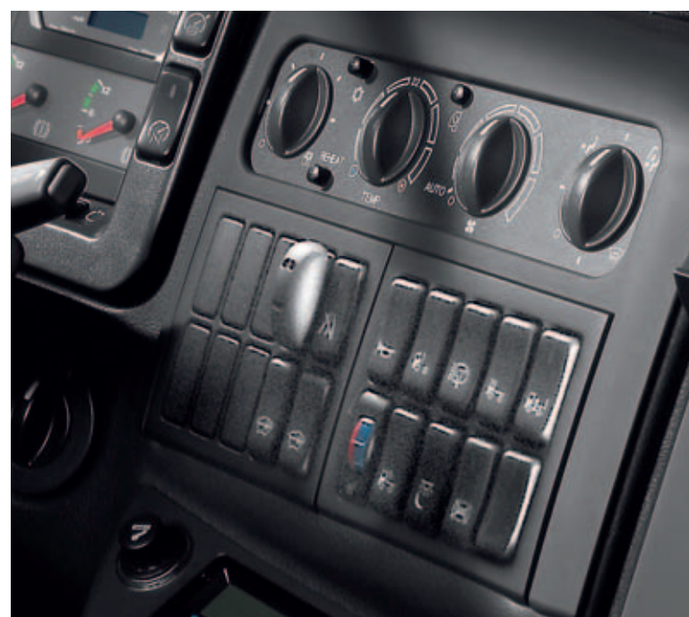
Air-conditioner with automatic temperature regulation.
