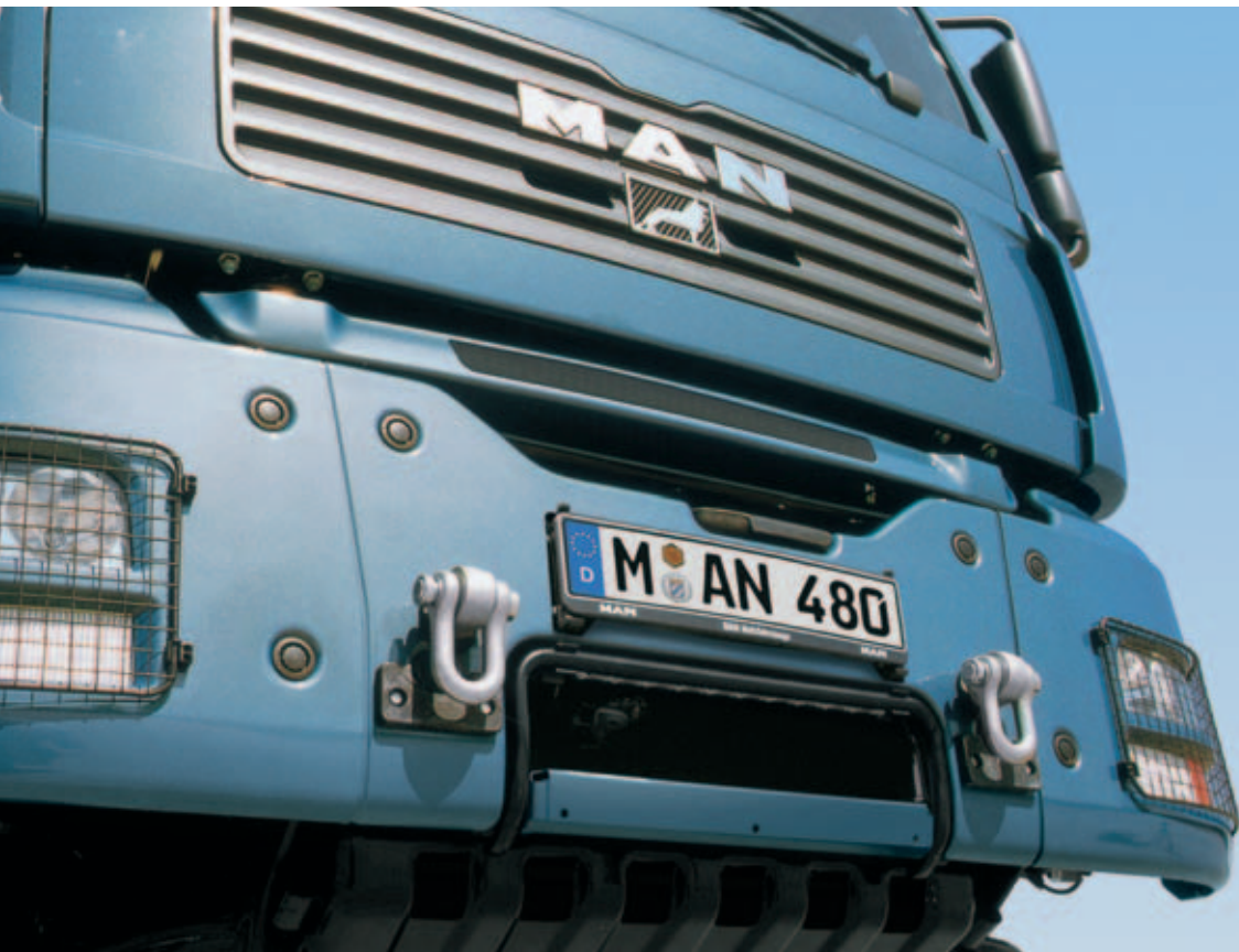
Three-piece steel bumper with central towing coupling.
