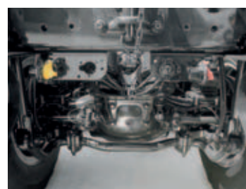
Planetary axle with high ground clearance.
