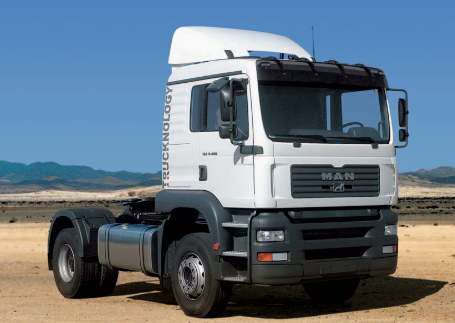
Semitrailer tractor 4x2 with leaf suspension.
