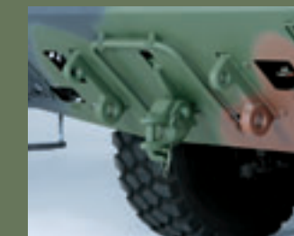
SX: Recovery equipment front
