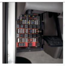
The T600's power distribution box puts all circuit protection elements – fuses, relays and breakers – in one quick-to-reach location.
