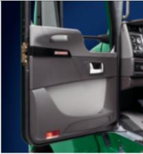
Available in Diamond (right) and Splendor (above) upholstery, Kenworth's new door pad presents a soft, durable, low-gloss luxurious finish you might associate with the finest automobiles. The new door pad design positions the window, door lock and mirror controls for easy touch access.
