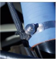
Huckbolts hold with six times the Constant torque hose clamps – standard on Kenworth trucks – go on tight and stay that way.
