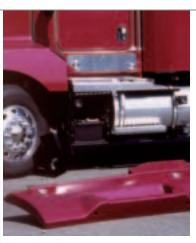
Servicing the battery system is easier on a fairing-equipped T600 than on most trucks. Only 5 bolts stand in the way of complete access.
