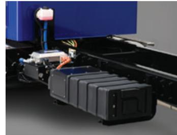
*High energy lithium ion battery and controls for fuel saving Eaton hybrid system.*
