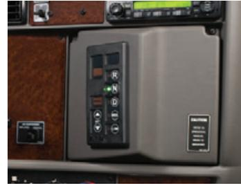
*Easy-to-operate dash control panel for Eaton automated and Allison automatic transmissions.*
