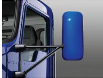
*Heated and electronically-adjusted aerodynamic mirrors.*
