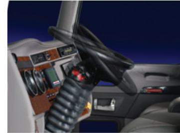
*Tilt and telescoping steering column.*
