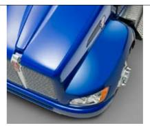
The four-piece hood and fenders are molded from Metton, a high-tech light weight composite material for added durability and repairability.
