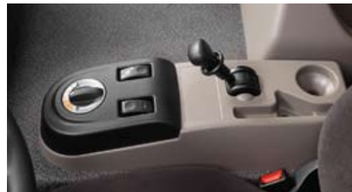
The AS-Tronic control panel is located on the console next to the driver's seat.
